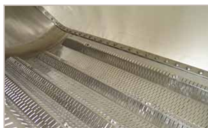
connected draining channels, electropolished
